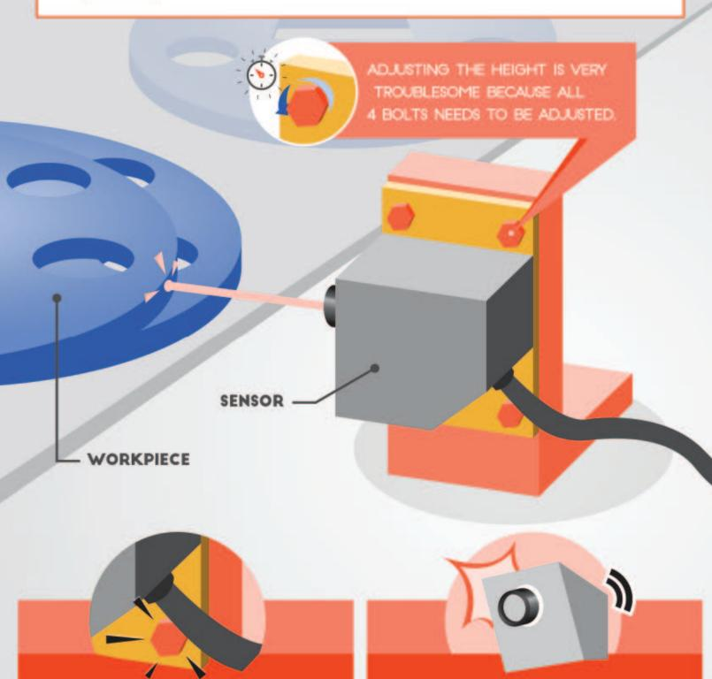
THE BOLTS UNDERNEATH THE SENSOR ARE DIFFICULT TO ACCESS AND MORE TIME TO REMOVE. TIGHTENING OF THE BOLTS CAN ACCIDENTALLY SHIFT THE HEIGHT OF THE SENSOR.
