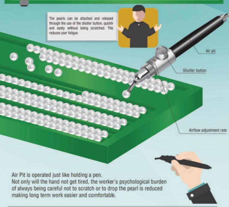
Appropriating tip attachments to suit the size of the pearls is also advised. Moreover, the strength of the suction force can also be controlled with the airflow adjustment screw, so large and heavy
