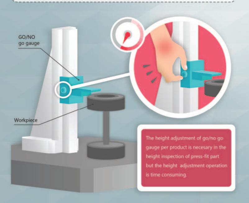
The adjusted gauge height is fixed by tightening the two screws but the aligned height is changed when the screws are tightened, in that case, the height adjustment needs to be repeated. If change product is frequent, the adjustment is very difficult.
