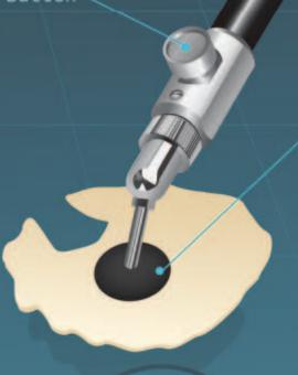
By placing the rubber pad type attachment close to the cracker, it will be gently absorbed avoiding any damage.
