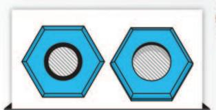
If the center of the workpiece deviates from below the lens even slightly, the image is distorted and accurate measurement is not possible.
