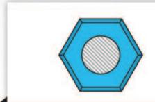
With the Telecentric Lens, image distortion is eliminated regardless of the workpiece's position - the hole's wall surface cannot be seen as well.
