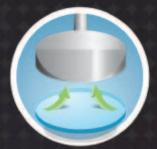
By placing the Spatula type attachment close to the mirror, the mirror will be gently absorbed avoiding any damage.
