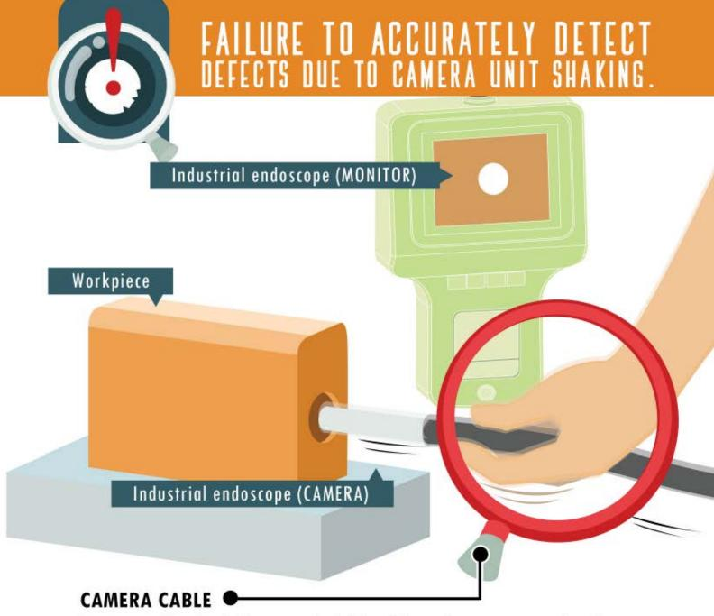
Is operated by hand. Because of shaking, blurry images are produced, givingway to possible overlooking of defects.
